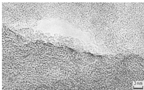
Figure 8 High-strength carbon fibre: (\text{NH}_4)_2\text{SO}_4 treatment (2 min, 1.72 V).
